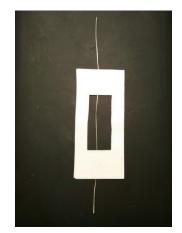
Figure 2. Banana fibre filament attached to a paper holder
