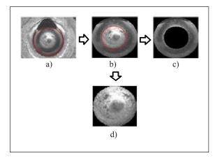
Figure 1. Extracted regions from the cartridge case image
