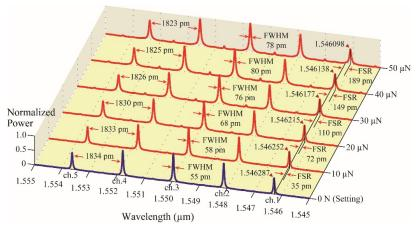
*Figure 3.* Simulation results of the comparing spectrum between the setting and sensing spectrum that can be obtained by the ring resonator system while exerting a force of 10  $\mu$ N, 20  $\mu$ N, 30  $\mu$ N, 40  $\mu$ N and 50  $\mu$ N on the sensing unit
