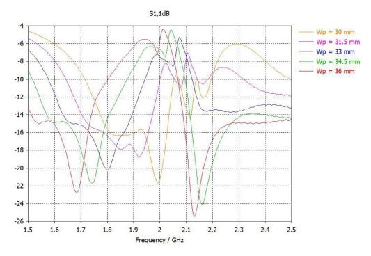
Figure 7. The simulation result of return loss for five different patch width values
