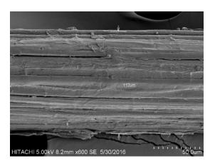
Figure 4a. SEM image of untreated banana fibre
