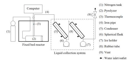
Figure 1. Experimental setup of pyrolysis
