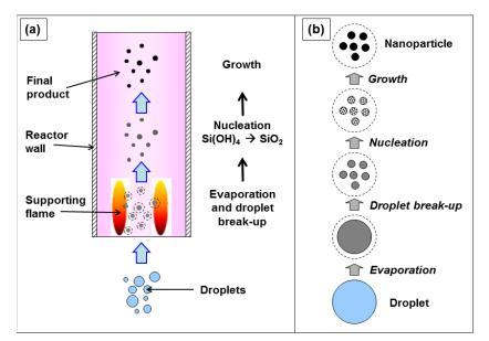
*Figure 2.* Illustration image of the particle formation mechanism. Figure (a) is the image for the particle travel phenomenon in the flame reactor, whereas Figure (b) is the particle formation mechanism
