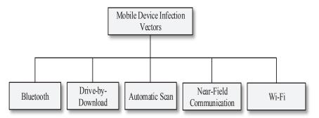
Figure 4. Mobile device infection vectors
