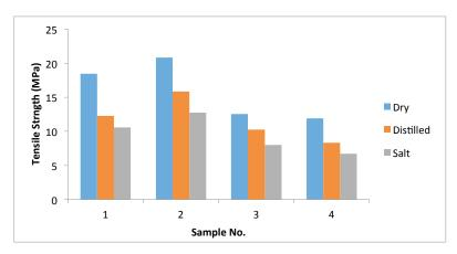
Figure 4. Tensile strength of composites
