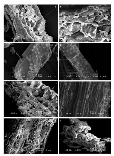
*Figure 1*. SEM image of (a) C before sorption, (b) C after sorption, (c) S before sorption, (d) S after sorption, (e) CG before sorption, (f) CG after sorption, (g) CM before sorption, (h) CM after sorption (× 1000)
