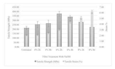
Figure 6a. Tensile strength and strain of untreated and treated single banana fibres
