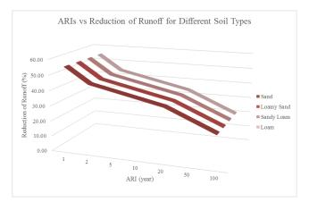
Figure 8. Reduction of runoff based on soil types and ARIs
