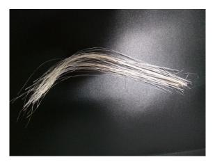
Figure 1. Untreated banana fibre in loose form
