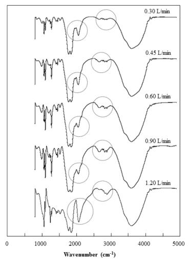
*Figure 8.* The FTIR analysis results of the samples produced at various LPG fuel flow rates in the range of 0.30 and 1.20 L/min. All the processes were conducted using a carrier gas flow rate (air) of 0.45 L/min, and a total air gas flow rate of 1.50 L/min
