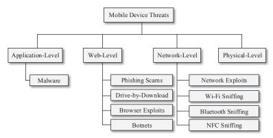
Figure 1. Threats to mobile device security
