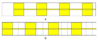
Figure 1. (a) Layout of collinear antenna, top view (b) Layout of collinear antenna, bottom view
