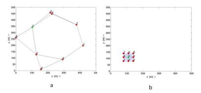
*Figure 2*. Random Topology (a) and Grid Topology (b) Every node is labeled with number. Both graph axes represent distance in metres. Red nodes represent dead node. Green nodes represent base station nodes
