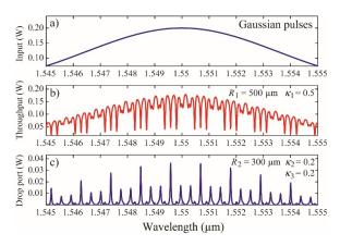
*Figure 2.* Simulation results with the obtained optical Vernier effects for a Gaussian pulse input of 10 nm bandwidth as a function of wavelength from 1.545 to 1.555  $\mu$ m
