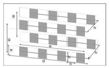
Figure 3. The Antenna MIMO design
