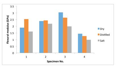
Figure 8. Flexural modulus of the composite
