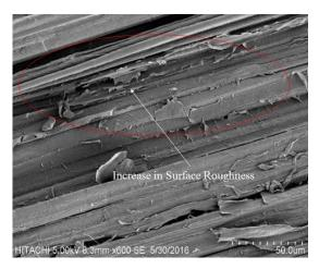
Figure 4b. SEM image of banana fibre treated with 6% NaOH for 2 hours
