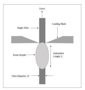
Figure 3. Schematic of the micro-droplet test
