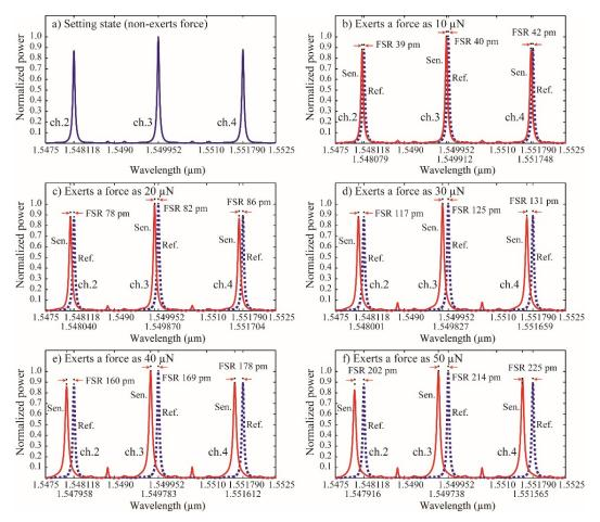
*Figure 4*. Simulation results of the comparing spectrum between the setting and sensing spectrum in channel 2, 3 and 4, a) for the setting state, b), c), d), e) and f), for a force exertion of 10  $\mu$ N, 20  $\mu$ N, 30  $\mu$ N, 40  $\mu$ N and 50  $\mu$ N, respectively
