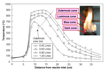
*Figure 6*. Reactor temperature profile at the centre of the reactor at various LPG fuel flow rates in the range of 0.45 and 1.20 L/min. The process was conducted using a carrier gas flow rate (air) of 0.45 L/min, and a total air gas flow rate of 1.50 L/min. Panelled figure was the photograph image of fire with information about the position of fire interface
