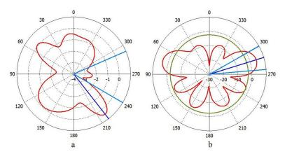
Figure 15. Radiation pattern of the antenna: (a) Azimuth plane, and (b) Elevation plane
