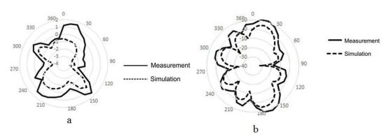
Figure 18. The result of measuring radiation pattern: (a) Azimuth plane (b) Elevation plane
