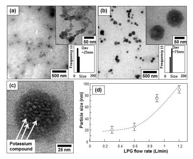
*Figure 7*. The TEM images of particles produced at various LPG flow rates. Figures (a) and (b) are the samples prepared at the LPG fuel flow rate of 0.60 and 0.90 L/min, respectively. Figure (c) is the high magnification of the TEM image of sample prepared at the fuel flow rate of 0.9 L/min. Figure (d) is the effect of LPG flow rate on the particle size. All the processes were conducted using a carrier gas flow rate (air) of 0.45 L/min, and a total air gas flow rate of 1.50 L/min
