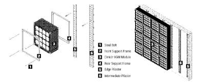
Figure 5. Elmich vertical greening modules (Elmich, 2008)
