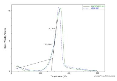
Figure 7b. TGA combustion temperature for treated and untreated fibres
