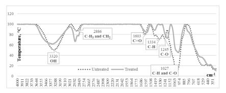
Figure 5. FTIR elements of treated and untreated fibres
