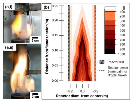
*Figure 5*. Photograph image of flame-supported pyrolysis method. Figures (a,i) and (a,ii) are the photograph images of flame produced using 0.45 and 1.20 L/min of LPG, respectively. Figure (b) is the reactor temperature profile at 0.90 L/min of LPG. All processes were conducted using a carrier gas flow rate (air) of 0.45 L/min, and a total air gas flow rate of 1.50 L/min
