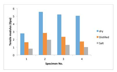
Figure 5. Tensile modulus of specimens
