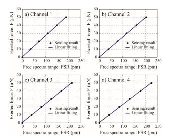
*Figure 5.* Linearity relation of the exerted forces as a function of free spectra range shifts in each considered channel
