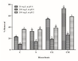
*Figure 2*. Biosorption efficiency of C, S, CG and CM in 20 mg/L Cr(VI) solution at pH 4 and 200 mg/L Cr(VI) solution at pH 2 and 4 (SD: 0.5 g, SR: 350 r/min, temperature:  $25^{\circ}$ C, CT: 24 h). Different letters indicate significant difference (p<0.05) between sorbents in the same MC and initial pH. Values are mean  $\pm$  SD (n=3)
