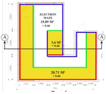
Figure 5. Detailed map of the electron maze chamber
