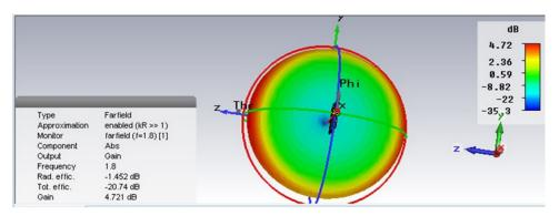
Figure 6. Gain and radiation pattern of the antenna at 1.8 GHz
